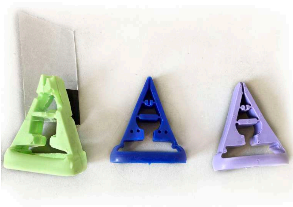
Figure 4.3: Multiple iterations of the tail with increasing hardness from left to right. (left) Body Double Silk; (middle) Dragon Skin 20; (right) Smooth Sil 945
