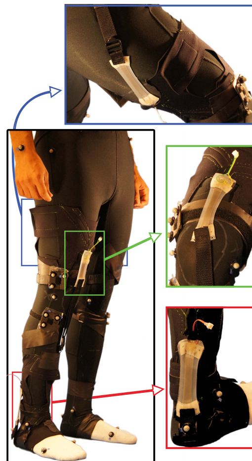
Fig. 2. A photograph of the prototype sensing suit worn by a participant. The call-outs show (from top to bottom): the hip sensor, the knee sensor and the ankle sensor.
